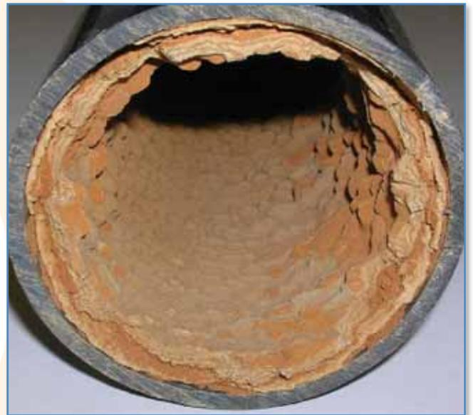
Loss of diameter due to an accumulation of lime
