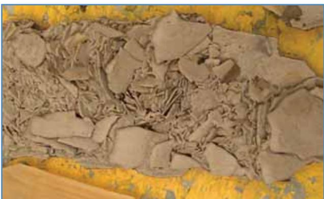
Remains of lime incrustation in a pipe not treated with ioncal
